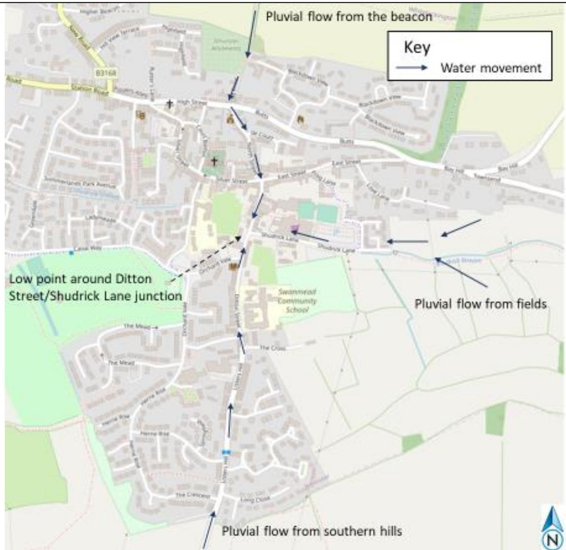
**Figure 29: Pluvial flows around east Ilminster**
